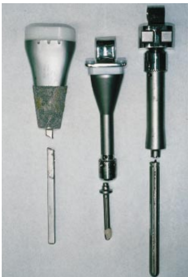
Figure 31.7 Various proximal tibial prostheses utilized during the 1980s showing a common mode of failure. The custom prosthesis on the left with porous coating shows stress fracture of the stem and similarly both expandable prostheses by different manufacturers show fracture of the stem. This was a common occurrence in the older design intramedullary stems that were often too short and narrow. In general, stems of greater than 9-mm are now utilized and rarely fracture.
