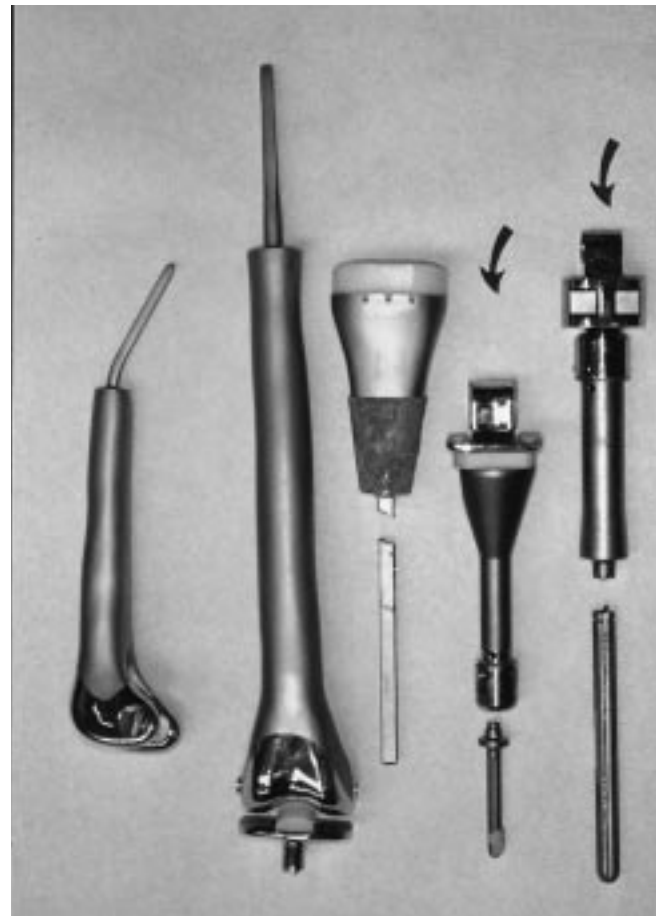
Figure 25.10 Composite photograph showing failures of several different prosthetic devices utilized during the 1980s and the various modes of failure. The most common mode of failure was either stem breakage or bending. Today, stems are heavily forged, have a curved transition at the junction with the prosthesis and are rarely less than 9 mm in diameter.
